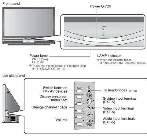
● Connecting terminals on the back of the TV ⇒ "Connecting External devices" (P. 10)
